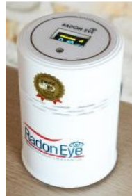
Figure 1. Ion chamber-type radon counter : RD200
